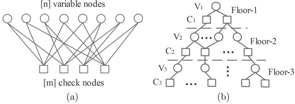
Figure 1: A bipartite graph in (a) and a tree expanded from a variable node in (b). The variable nodes and check nodes are represented with circles and squares, respectively.
