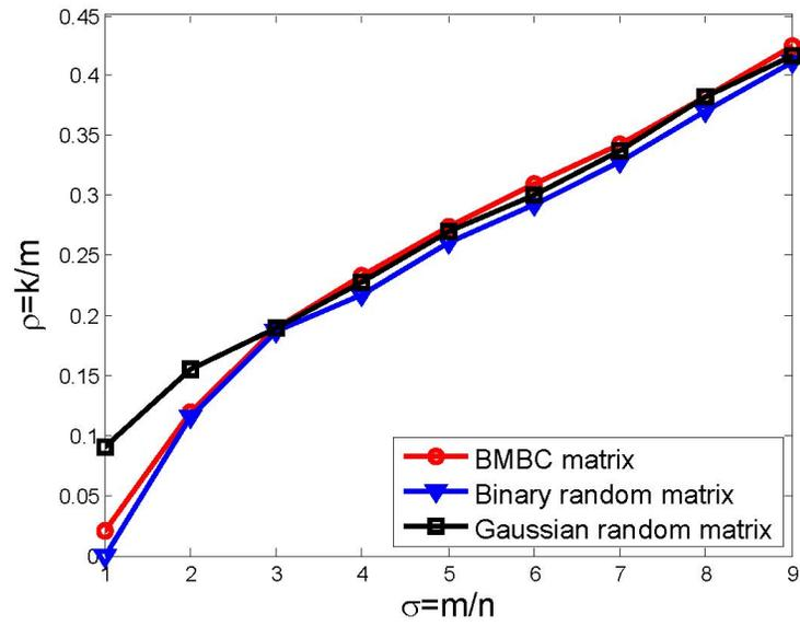
Figure 3: The guaranteed sparsity  $k$  (depicted with  $\rho = k/m$ ) of three types of matrices with varying compression ratios  $\sigma = m/n$ ,  $n = 1000$ . Note the BMBC matrix and binary random matrix share the same column degree as detailed in Table 2.
