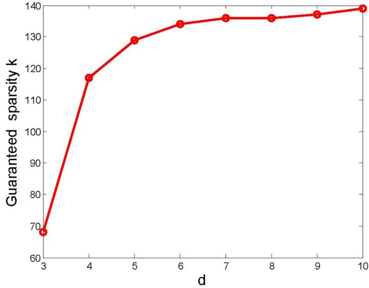
Figure 2: The guaranteed sparsity  $k$  of  $500 \times 1000$  BMBC matrix with column degree  $d$ .
